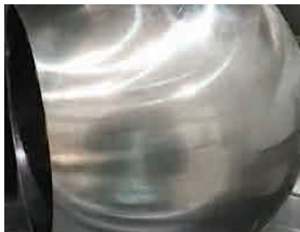
Surface mirror level finishing Ra \leq 0.4 \mu m
